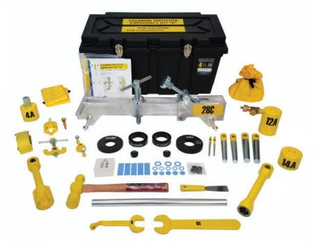
The Chlorine Institute Emergency Kit "B" is manufactured to the design specifications of the Chlorine Institute. The Emergency Kit "B" contains devices to stop leaks at the valves, fusible plugs, and in the side wall of chlorine one ton containers which conform to specification DOT 106A500X & DOT 106A500W. Two instruction booklets explaining the application of each device are included. An instruction DVD for Kit B is also available.
